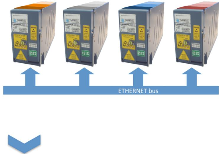
**Multiplex communication bus reduces the amount of wiring and provides complete communication flexibility**
